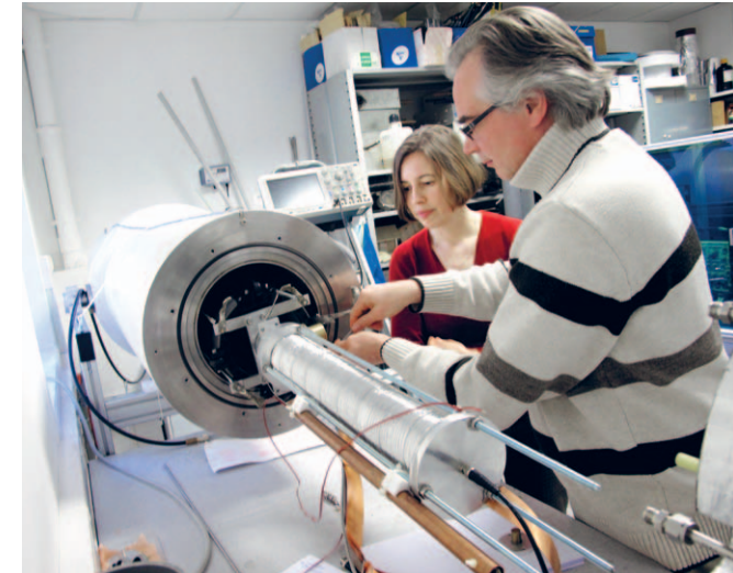
Researchers are examining the samples for the space charge test of the insulation.
